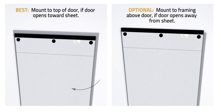
Proper placement on door should cover gaps all around door frame as illustrated below. To seal off gaps around the door, add an Audimute Acoustic Door Seal Kit.
